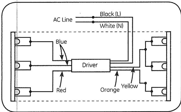
**4C Three Tube Fixture:** Connect the black (L) and white (N) wires of driver to black and white wires of AC line, respectively. Connect the two blue wires of the driver to one set of lampholders at one end. At the same end connect one red wire to remaining lampholder. At the opposite end, connect yellow wire to the lampholders of the corresponding blue wires. Connect orange wire to the remaining socket (opposite to red wire connection). Cap remaining red wire.
