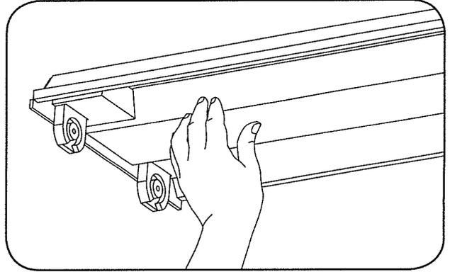
**6A** Compact wires and reattach fixture coverplate.
