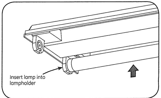
**7** Insert the energy smart® LED tube into the lampholder of the fixture and rotate 90 degrees. Repeat for remaining tubes.
