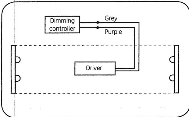
**5 Dimming option:** Connect the grey and purple wires from the driver to the dimming controller (If not dimming, individually cap wires).
