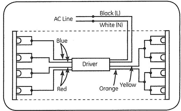
**4D Four Tube Fixture:** Connect the black (L) and white (N) wires of driver to black and white wires of AC line, respectively. Connect the blue wires of the driver to one set of lampholders at one end. At the same end connect the red wires to other set of lampholders. At the opposite end, connect yellow wires to lampholders of the corresponding blue wires. Connect the orange wires to the corresponding lampholders of the red wires.
